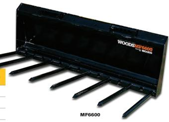
Sturdy reinforced design ensures extra strength, and replaceable, heat-treated round tines provide a working length of 25.5-inches. For applications requiring tighter spacing, these forks will accept up to nine additional tines.
