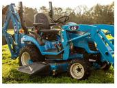
60 Inch Mower Deck Heavy-Duty Mower Deck Provides An Excellent Cut And Makes Use Of The Standard Mid-PTO
