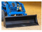
Deluxe Loader 2 Lever Skid Steer Coupler Allows For Universal Skid Steer Attachments
