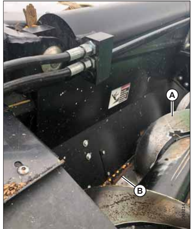
Figure 5.11: Auger-to-Stripper Bar Clearance
