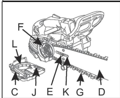
7. Install Bar/Clutch Cover (C) over Guide Bar Stud (H). Make sure chain tension Adjuster Pin (J) fits into the Guide Bar Adjuster Slot (K), and Brake Band (L) is positioned around Clutch Drum (M). Tighten Bar/Clutch Cover Nut (B) finger tight.
