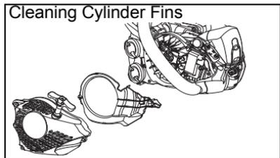
2. Use compressed air or wooden tool to remove dirt and dust from between fins to let cooling air pass easily.
