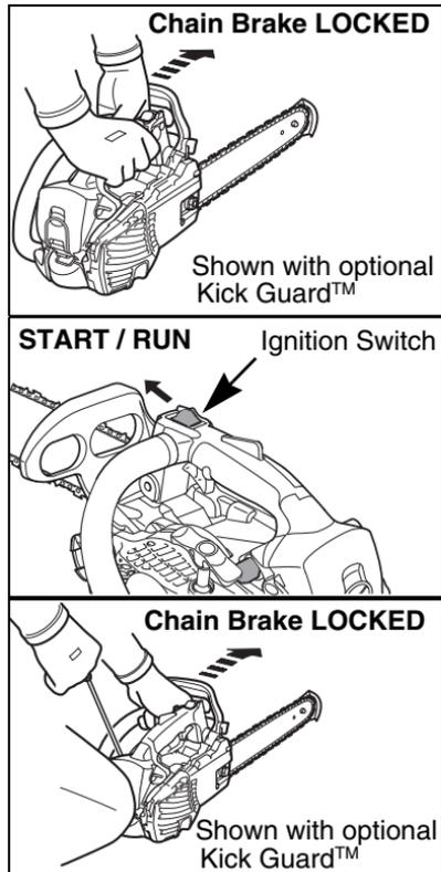
5. Choke may be used if necessary, but after first starting sound, squeeze throttle trigger to release choke and return engine to idle.
