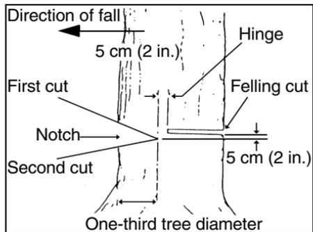
between the notch cut and felling cut about 5 cm (2 in.) will act as a hinge when the tree falls, guiding it in the desired direction. When the tree starts to fall, kill the engine, place the saw on the ground and make your retreat quickly.
