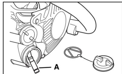
1. Pull Oil Filter out through oil port, and inspect Oil Filter.
