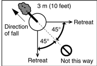
Begin the cut on the side to which the tree is to fall. Cut a notch about 1/3 of the way into the tree. The position of this notch is important since the tree will try to fall "into" the notch. The felling cut is made on the side opposite the notch and at a level about 5 cm (2 in.) above the bottom of the notch. Do not try to cut through to the notch with the felling cut. The remaining wood between the notch cut and felling cut
