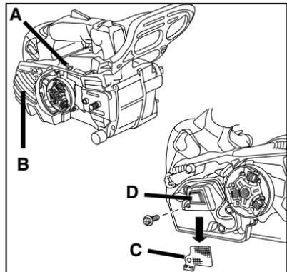
Note: When cleaning carbon deposit, be careful not to damage the catalytic element inside Muffler Body (D).
