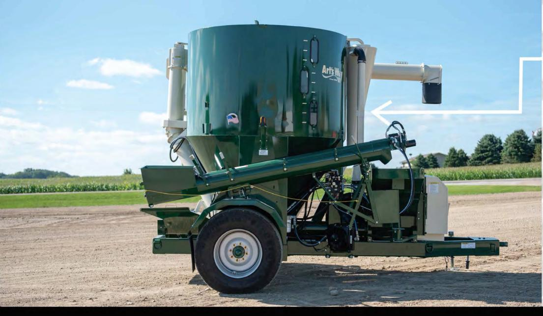
Largest US Grinder Mixer! The 8215 Grinder Mixer was built to withstand the test of time and bring ease to your farm. This large 215 bushel mixing tank is paired with a 26 inch hammer mill for powerful and efficient feed processing. The self-contained hydraulics allow for a more hands free environment.
