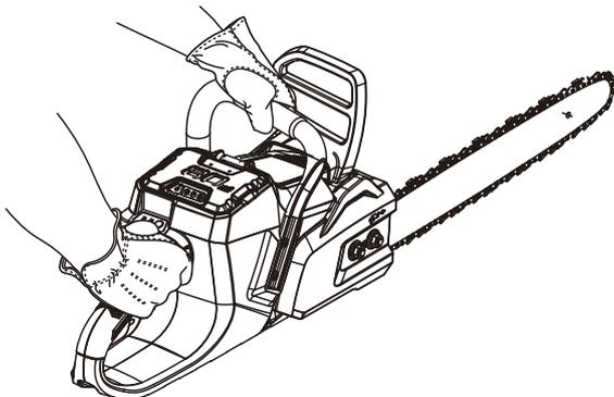
1. Hold the chainsaw with your right hand on the rear handle and left hand on the front handle.
