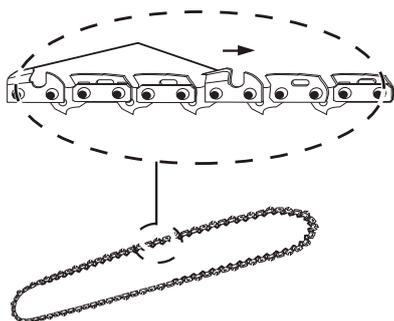
5. Put the chain in position and make sure that the loop is behind the guide bar.
