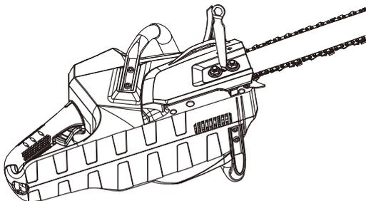
5. When the chain is at the wanted tension, tighten the lock nuts.
