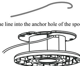
4. Wind the cutting line around the spool tightly in the indicated direction.
