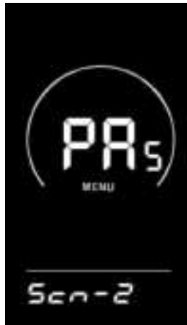
Fig. 8-7 Assistance sensor sensitivity setting interface
