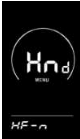
Fig. 8-11 Handlebar Assist Level Enable Setting Interface
