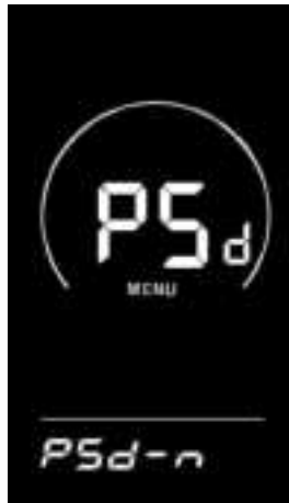
Fig. 8-15 Password Enable Confirmation Interface
