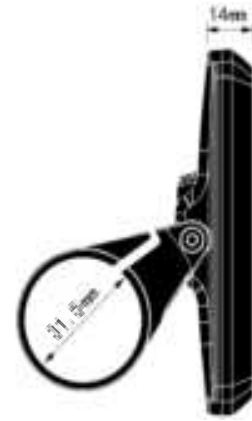
Fig. 3-4 Side View of Display Dimensions
