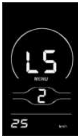
Fig. 7-2 Speed Limit Setting Interface
