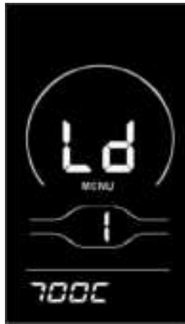
Fig. 7-1 Wheel Diameter Setting Interface
