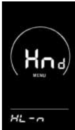
Fig. 8-10 Handlebar Push Assistance Setting Interface
