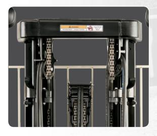
Hi-Vis™2 mast assembly - Designed to be durable and long-lasting, while requiring minimal adjustments and maintenance, even in demanding applications with captive-load attachments. Hose take-ups and lift mechanisms are designed to last, yet allow easy servicing for minimal downtime. Sectioned hoses can be repaired without changing the entire hose, and unique sheaves allow larger radius bends which prevent kinking.
