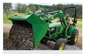
OPTIONAL 300E LOADER with a Mechancial Self Leveling Loader (MSL) option has a lift height of 84 in. (214 cm) and a lift capacity of 1283 lb (539 kg) measure at 19.7 in (500 mm) ahead of the pivot, so you can shoulder just about anything. Non Self-Leveling option available.
