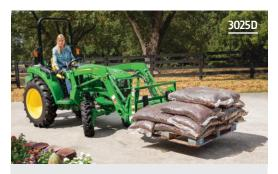
63.6 IN (161.5 CM) TURNING RADIUS. As measured from the inner rear tire with a 300E loader. To maneuver around tight spaces. Add optional pallet forks for even more versatility.
