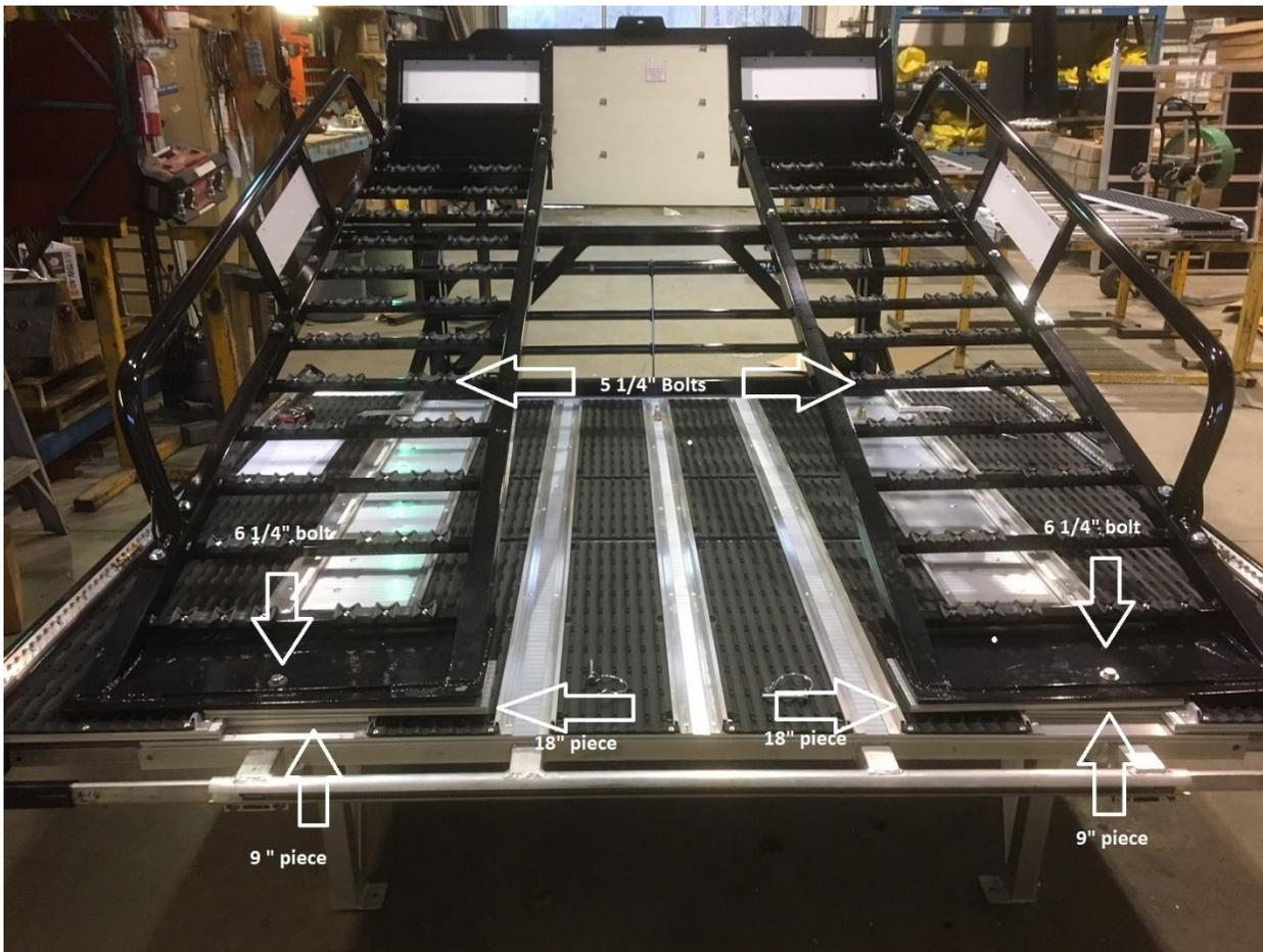
4. Install 2 – 6 1/4" bolts with 2 flat washers and nylocs. Thru the deck pad as well as the 18" and 9" spacers and thru the deck.
