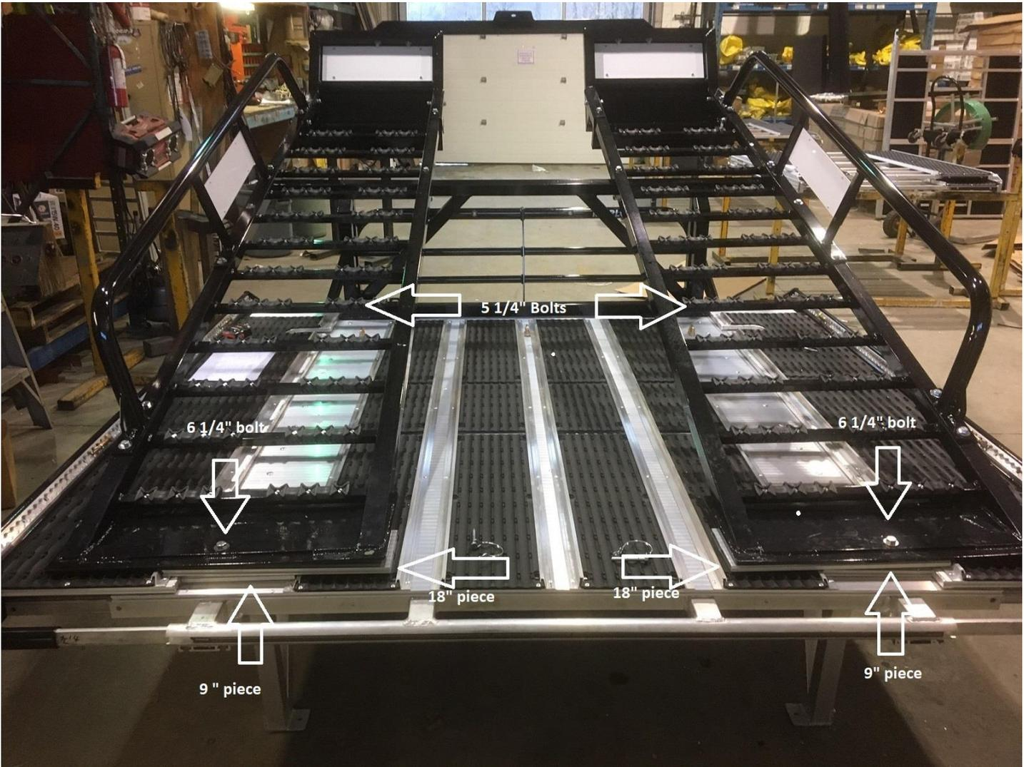
7. Attach side rail bars with 14 – 3 1/4" bolts with washers and nyloc nuts (do not tighten).
