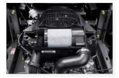
**ENCLOSED CANISTER AIR FILTER**
