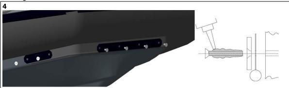
Place the buoyancy tube and make fast the outer flap (buoyancy tube deflated) using the stainless steel bars and the screws supplied in the buoyancy tube kit. To ensure that the assembly is mechanically secure, apply medium strength threadlocker to the screws.
