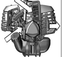
Dust and grass build up on the outside of the cylinder. This build up insulates the engine and prevents the heat from leaving.
