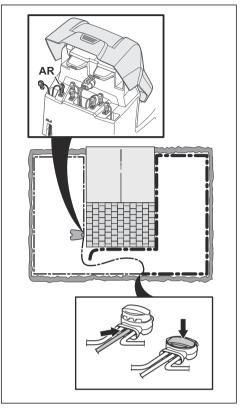
If the indicator lamp now is green, then the break is somewhere in the wire between the disconnected end to the point where the new wire is connected (thick black line below). In that case, move the connection for the new wire closer to the disconnected end (roughly at the middle of the suspected wire section) and check again if the indicator lamp is green.
