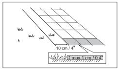
If you have a paving stone path that is in level with the lawn, put the boundary wire below the paving stone.
