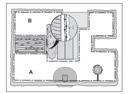
Put the boundary wire around the secondary area (B) to make an island. Refer to To make an island on page 16.
