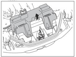
Disconnect the battery cable from the main circuit board.
