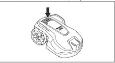
Push the **ON/OFF** button for 3 seconds and make sure the product is switched off. Check that the indicator lamp on the keypad is not lit. This means that the product is disabled. Refer to *To use the ON/OFF button on page 31*.
