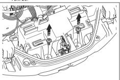
Push to detach the clips and lift up the battery holder.
