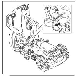
**Note:** Make sure the that the grommets for the charging cable are correctly installed to seal against moisture after you remove the body of the product.
