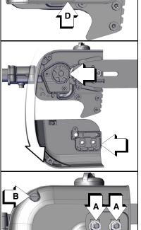
Hold the bar nose up. Install 4. guide bar cover (D). Install the guide bar nuts (A). Tighten the rear nut first, then tighten the front nut. Install and tighten the guide bar cover screw (B)
