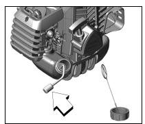
When the inside of the fuel tank is dirty, rinse the tank out with C. gasoline to clean it.
