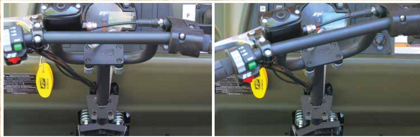
By adding a spring element between the handlebars and the brake system we achieved a progressive dual-rate steering system.
