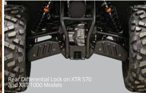
Rear Differential Lock on XTR 570 and XRT 1000 Models
