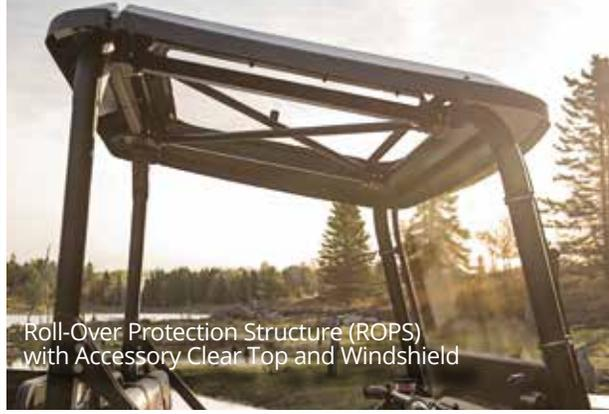
Roll-Over Protection Structure (ROPS) with Accessory Clear Top and Windshield
