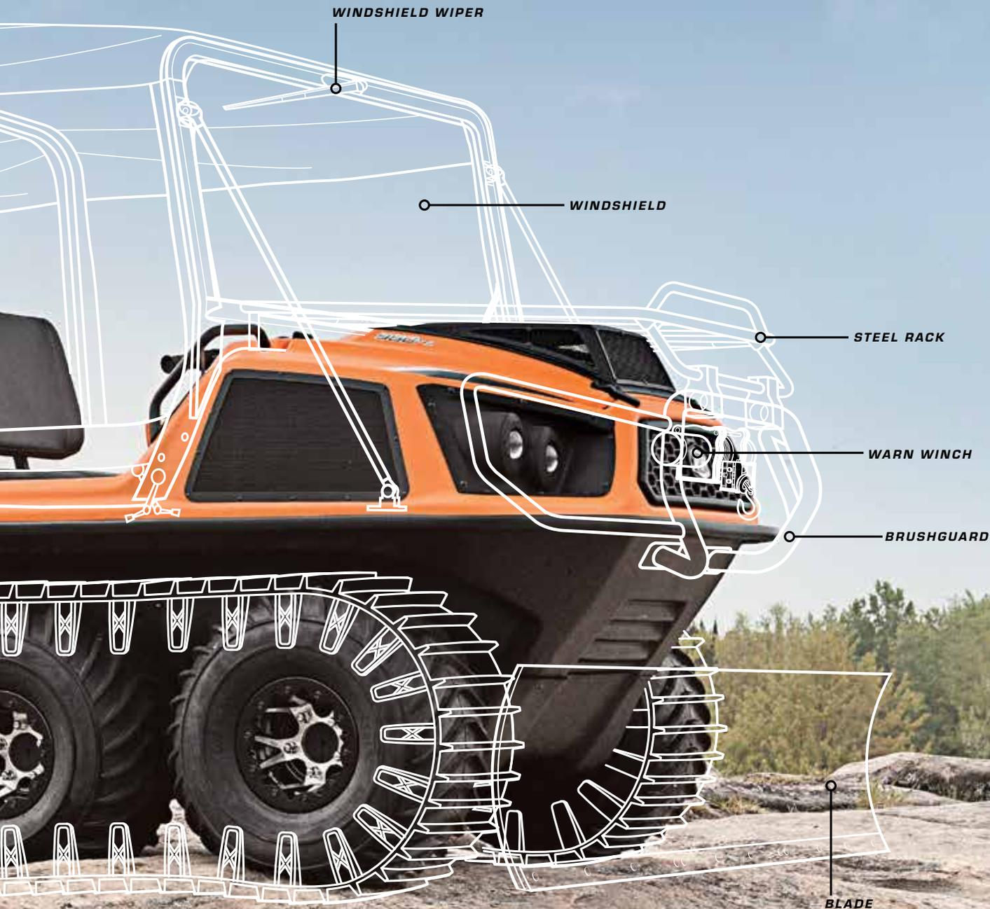
**Windshield** – Scratch-resistant acrylic means your windshield can take a beating out in the wild. Fold-over hinge for storage and a mounting location for optional windshield wiper accessory make installation quick and easy.
