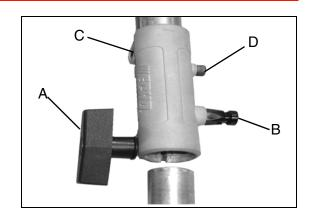
4. Remove coupler (E) from upper drive shaft assembly by loosening clamping screw (C) and removing set screw (D).
