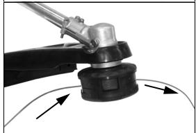
4. Hold trimmer head while turning knob clockwise to wind line onto spool until about 13 cm (5 in.) of each line remains exposed.
