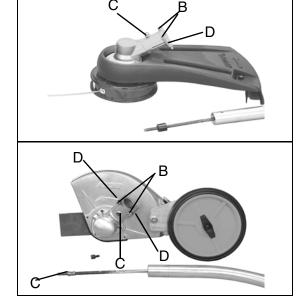
4. Install the gear housing and shield assembly.
