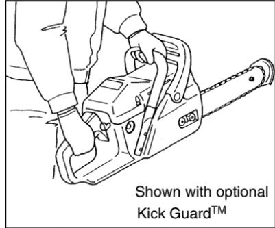
Start the engine, see that it is running properly. Squeeze the trigger to open the throttle wide open and start the cut. If the chain is properly sharpened, the cutting should be relatively effortless. It is not necessary to press down hard to make the saw cut. Pushing the saw too hard will slow the engine and cutting will actually be more difficult.
