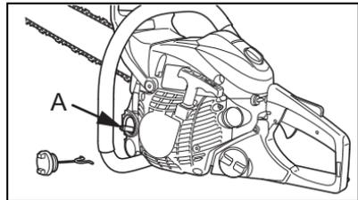
1. Pull filter out through oil port, and inspect filter.
