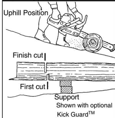
Keep in mind that the wood is heavy and that it will bend and pinch the saw if improperly supported. The trunk will weaken at the point where you make the cut unless the tree is lying on perfectly flat ground or supported as shown. If you make the cut with the tree on the ground, don't let the saw's chain dig into the earth; it is harmful for the saw, and you stand a good chance of being struck by flying debris.
