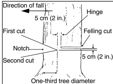
To fell big trees with a diameter exceeding twice the bar length, start the notching cuts from one side and draw the saw through to the other side of the notch. Start the back cut on one side of the tree, pivoting the saw through to form the desired hinge on that side. Then remove the saw for the second cut. Insert the saw in the first cut, very carefully so as not to cause kickback. The final cut is made by drawing the saw forward in the cut to reach the hinge.
