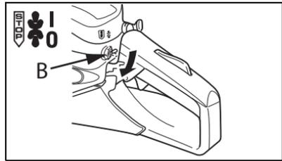
Note: If engine does not stop, pull choke control knob out fully to stop engine.
