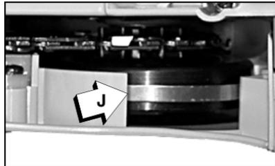
8. Adjust saw chain tension, as instructed in “Adjustment, Chain Tension”.
