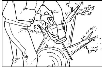
Don't cut with the saw overhead or aligned vertically with your body. If the saw should kickback, you may not have enough control to prevent possible injury.
