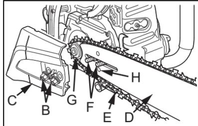
5. Mount guide bar (D) on studs (F) and slide toward clutch drum sprocket (G) to make saw chain (E) installation easier. Install saw chain around clutch drum sprocket and guide bar as shown, with cutters on top of guide bar facing forward.
