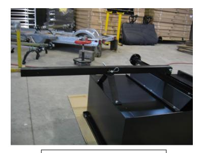
7. Attach coupler to the end of the tongue using two bolts.
