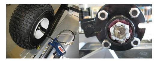
9. Inflate tires to the correct PSI & install on hubs, tighten with lug nuts. Then place water around the rim to check the bead for air leaks.
