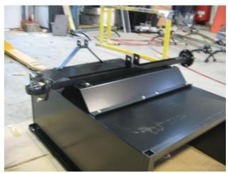
5. Attach axel to axel plate and bolt down tight.
