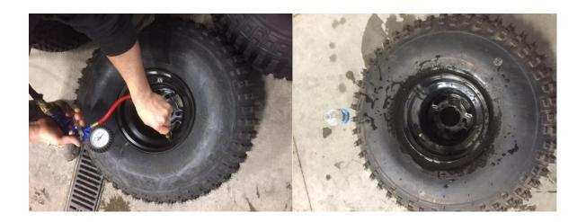
10. If you notice air bubbles you may have a slow leak. Take the tire and bounce it on even ground and test the rim once again with water to make sure the bead has sealed around the rim properly. Make sure to check both sides of the tire.
