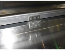
8. Place & mark holes for clip above inner stake pocket on left side of the trailer punch and drill as before.
