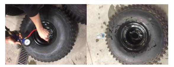
7. If you notice air bubbles you may have a slow leak. Take the tire and bounce it on even ground and test the rim once again with water to make sure the bead has sealed around the rim properly. Make sure to check both sides of the tire.
