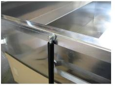
14. Mark & drill a hole for the top of the shock hinge from the hinged side of lid measure 26" from inside. Punch drill & install.
