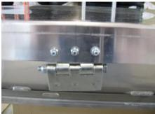
5. Center lid to trailer measure and mark for hinge holes on side of trailer.
