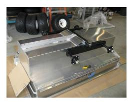
2. Place tongue in channel on bottom. Line up holes place 1-11mmx80mm bolt with a washer on both sides in hole. Place 1-18 mm Nylock nut on & tighten.
