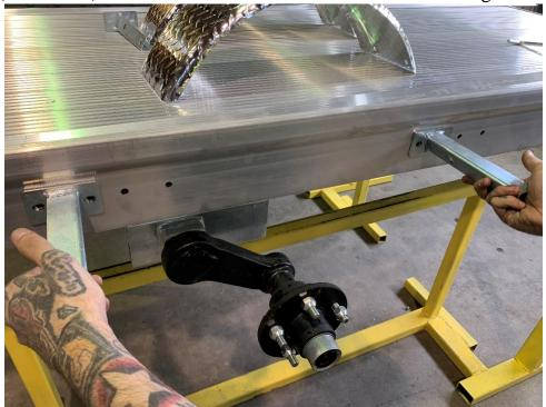
5. Mount the fenders to the fender brackets using the 20 x 7mm bolts. Make sure the bracket orientation matches the picture below.
