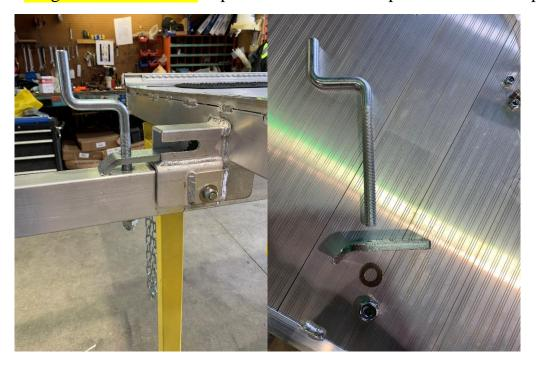
7. Attach the coupler to the tongue and the safety chains at the same time. Use the coupler mounting bolts, 80 x 10mm. The center link of the safety chain slides through the front bolt. Torque to 95 ft/lbs.
