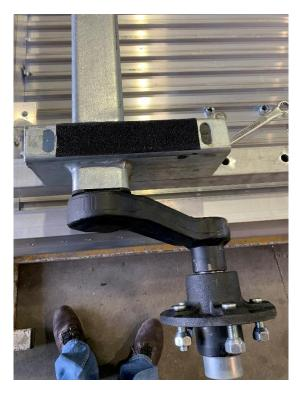
2. Bolt the axle to trailer frame 180 x 10mm bolts, washers and nylocks. Torque to 75 ft/lbs of pressure.
