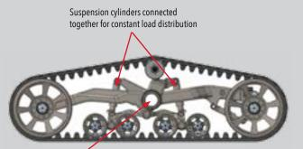
Note how the grain cart axle is stable as each track axle goes over the bump
