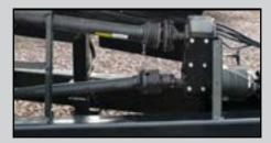
**PTO DRIVEN DRIVETRAIN** Gearbox includes 20" horizontal drag and 22" diameter vertical
