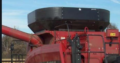
Since 1996, Demco Manufacturing has distributed this Stewart Steel product through our dealership network. Quality engineered and built to provide years of service, extenders offer the ability to extend the unloading auger to allow for greater clearance between the header and cart.
