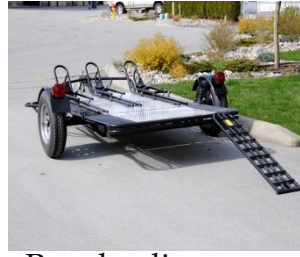
Rear loading ramp.
