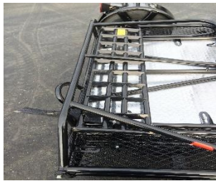
Loading ramp is bolted to underside.
