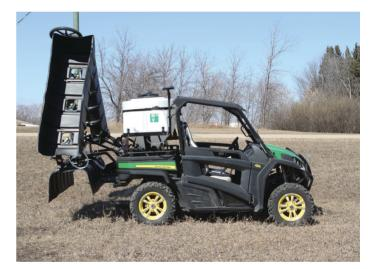
Ag Shield booms fold easily and lock for transport. You can load it on a trailer or in the back of a pickup truck for longer moves.
