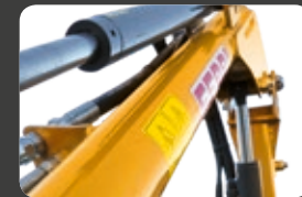
Circular section of the arms High Torsion Resistance.
