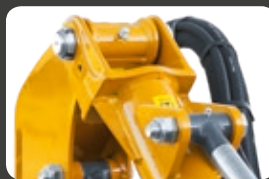
Drop forged parts for arm linkages.
