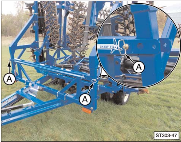
(A) Side Wing Lock Pins (enlargement shows pins in the storage location).
