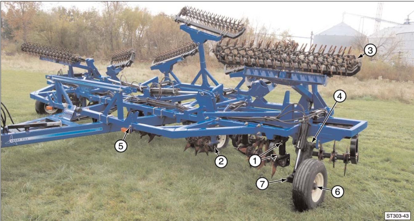
Model ST303 Shown. Models without side wings will not have pivot Zerk fittings (5). Refer to the Maintenance/Lubrication Chart for Item, Service, Quantity, and Frequency Information.
