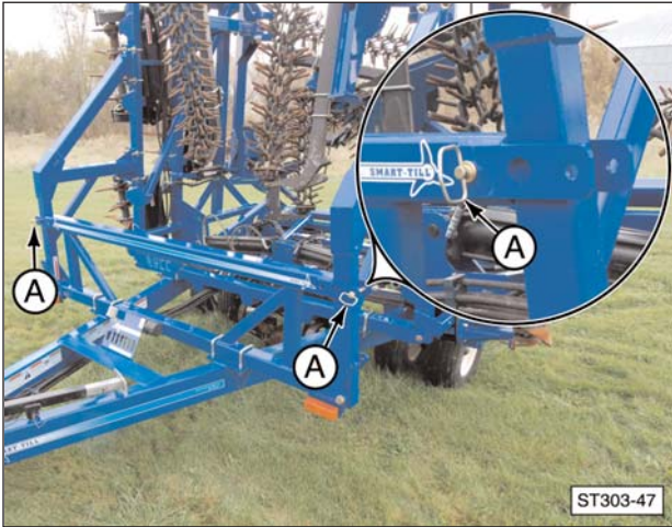
(A) Side Wing Lock Pins (enlargement shows the lock pin in the storage location).
