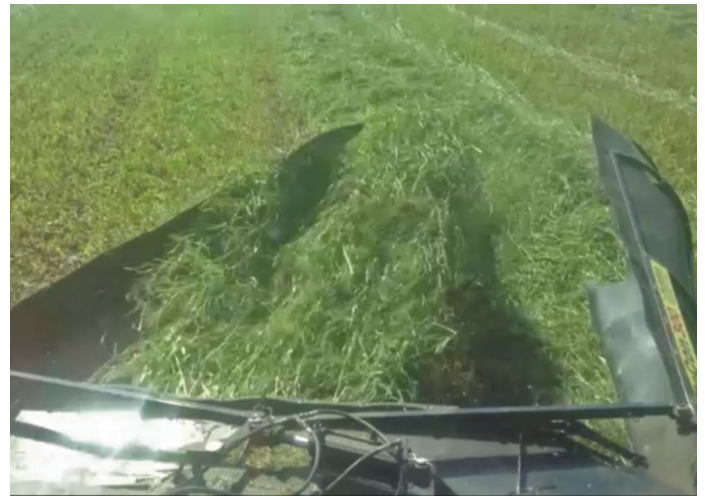
Side deflectors invert and move the swath onto dry ground to speed up the drying process and at the same time adjusting swath width to match baler.
