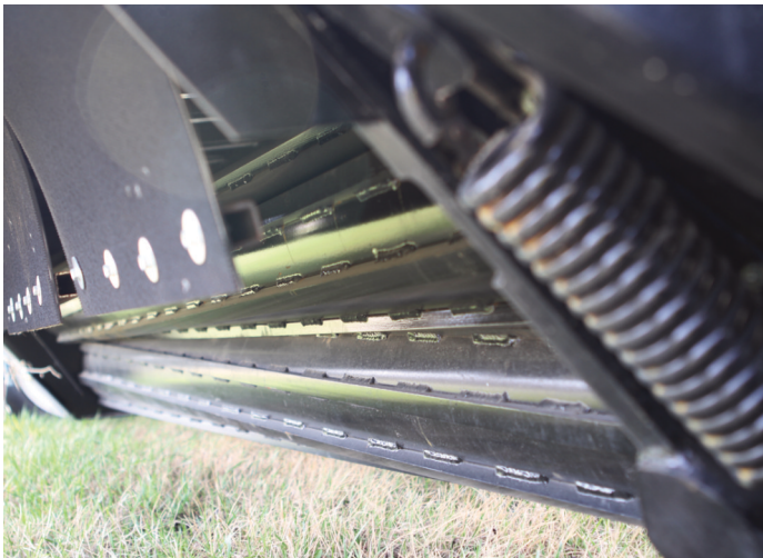
Precision timed and lathed rollers combined with hydraulic pressure opens stems fast and efficiently on all types of forage and cereal crops.
