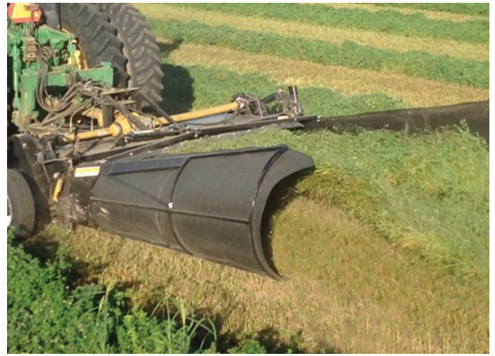
Recon 400 - 3 point hitch has a pivoting body that allows you to angle the machine 25 degrees to combine two swaths to save a raking pass.
