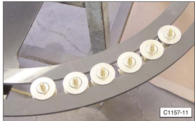
(12) Ball Bearing Roller.
