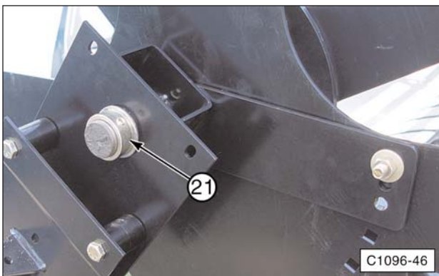
(21) Lock ring With Set Screws.
