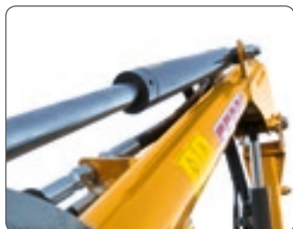
Bracci a sezione circolare High Torsion Resistance Arm with circular section H.T.R. (High Torsion Resistance)
