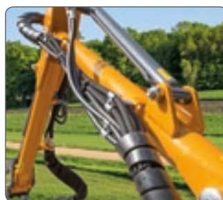
Bracci a sezione circolare High Torsion Resistance. Arms with circular section H.T.R. (High Torsion Resistance).
