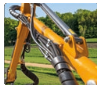
Bracci a sezione circolare High Torsion Resistance. Arms with circular section H.T.R. (High Torsion Resistance).
