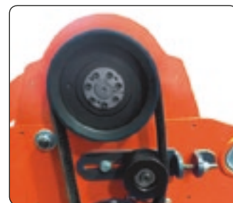
Trasmissione a 4 o 5 cinghie con galoppino flottante. Belt drive with 4 or 5 belts and tightening pulley.
