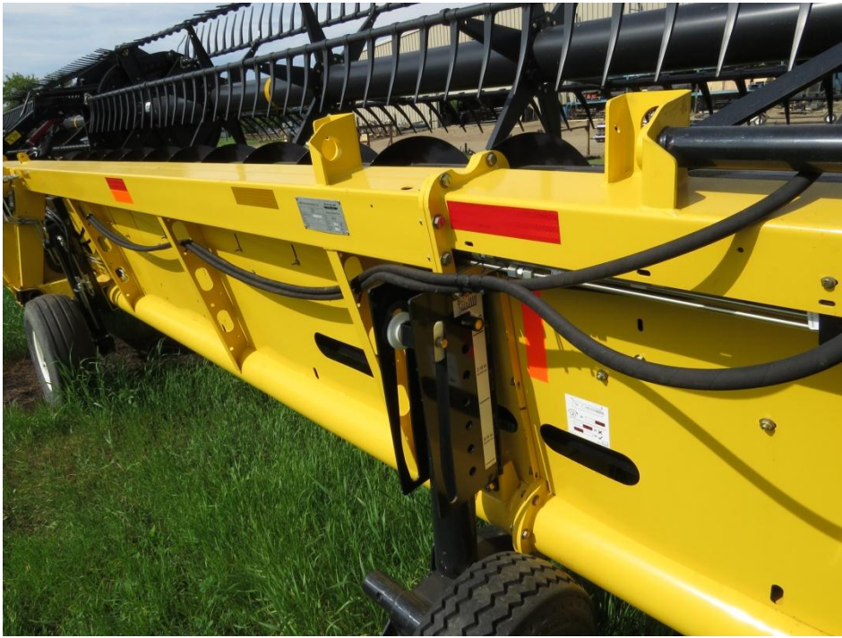
Run the hoses through the slots in the back of the header
