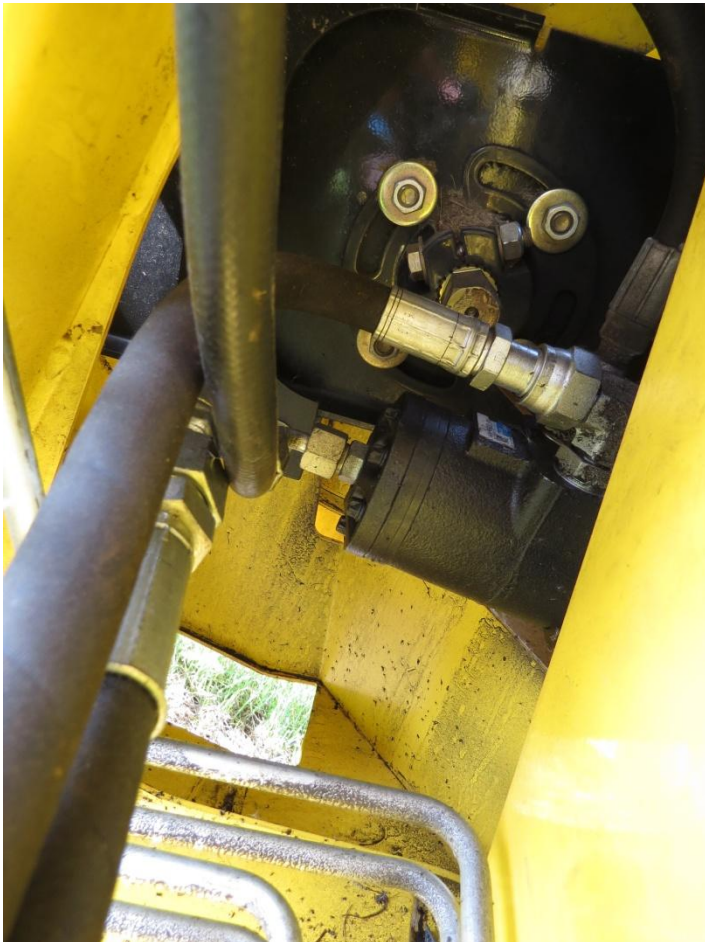
Ag shield fitting onto the return port of the canvas motor. Ag shield fitting to the hose that was removed from the return port on the canvas motor.
