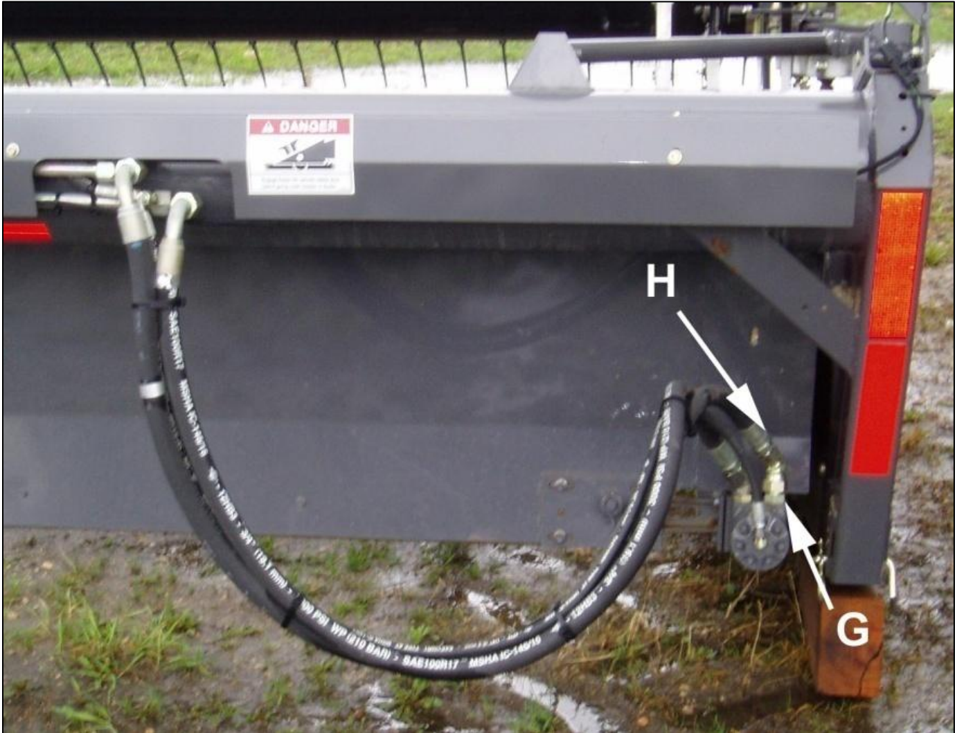
FIGURE 13 HOSES ON HEADERS WITH RIGHT HAND DRIVE CROSS AUGERS
