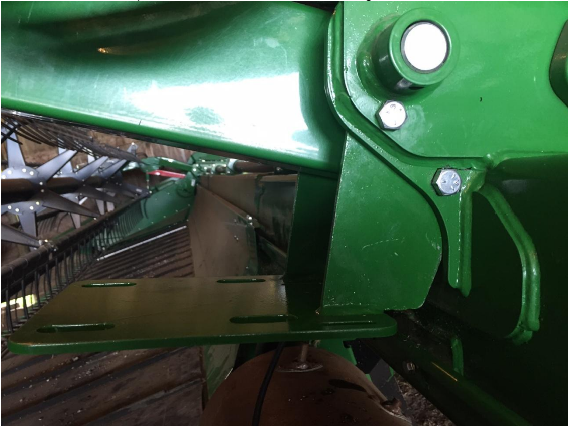
Photo of drilled and bolted mount plate.
