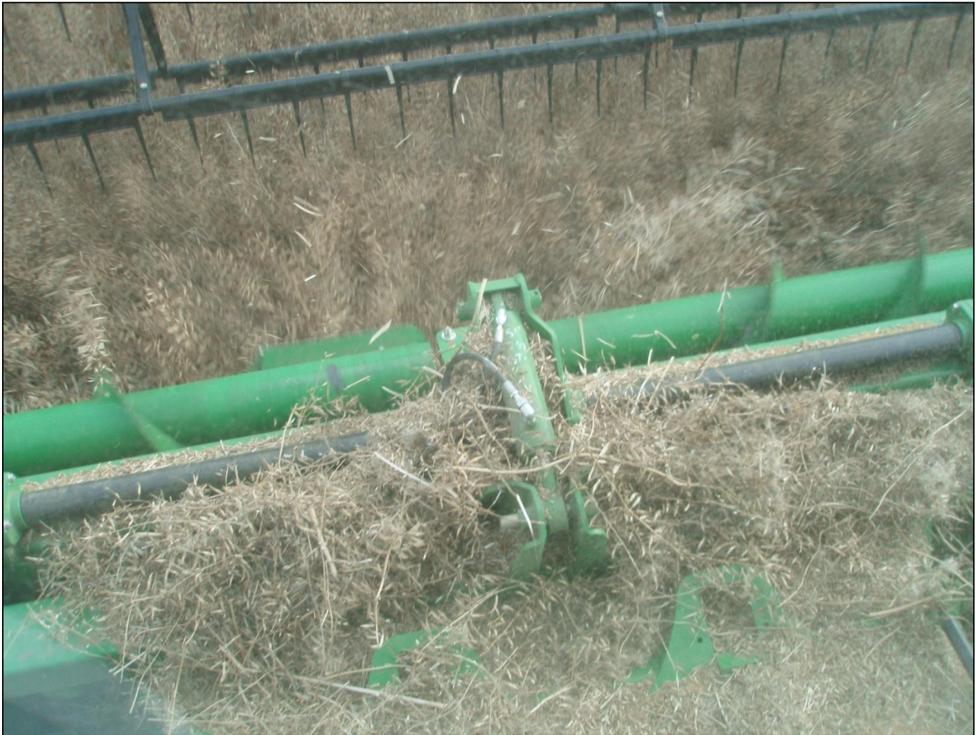
FIGURE 2 MUSTARD SHOWN BEING PULLED INTO THE CENTER OF HEADER
