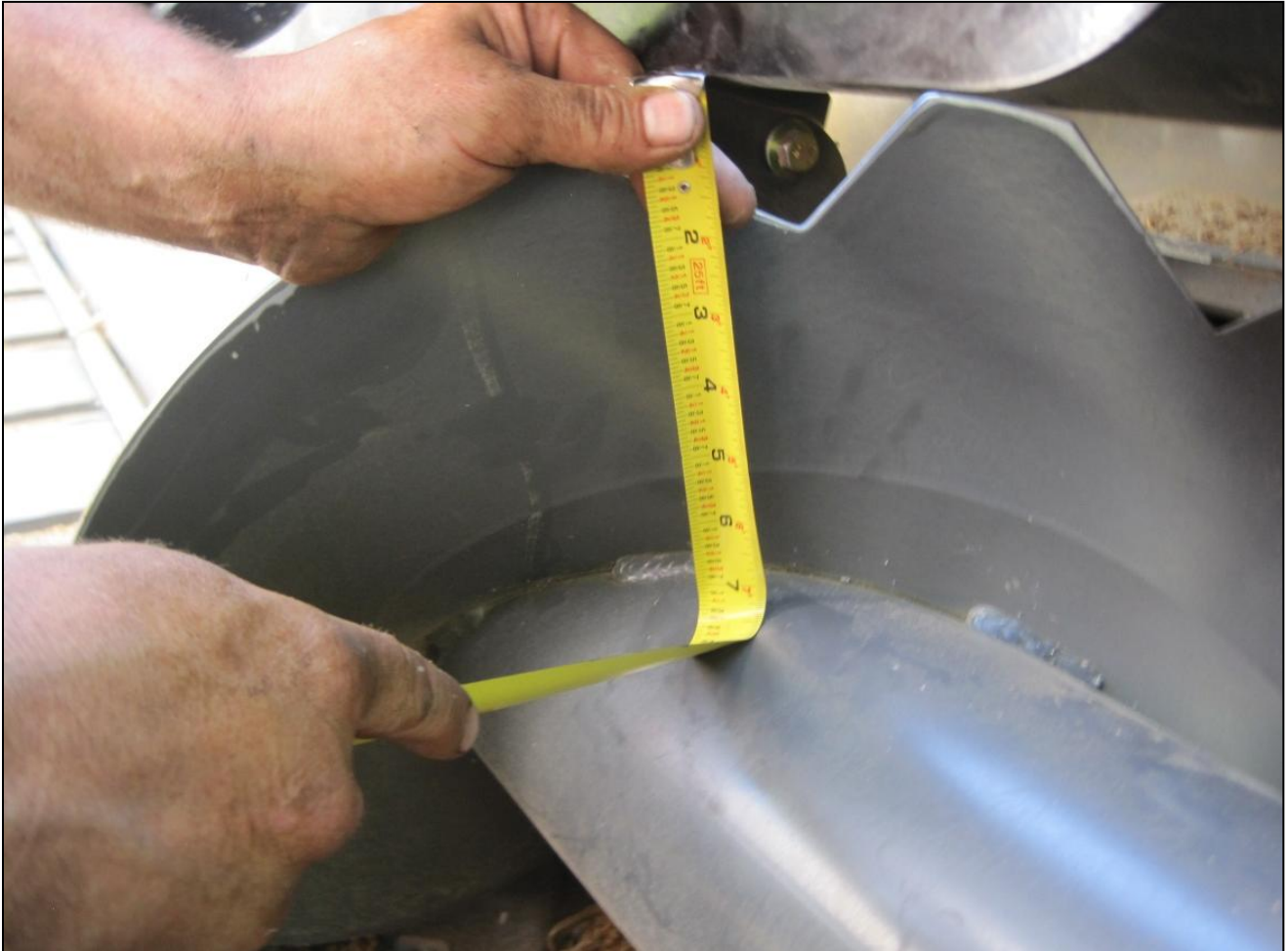
FIGURE 10 ADJUST UNTIL 7.25 INCHES BETWEEN 2 AUGERS AS SHOWN
