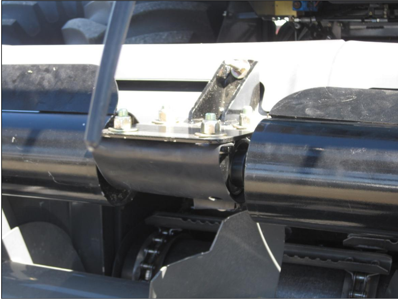
FIGURE 13 INSTALL PLASTIC CENTER COVER OVER THE BEARINGS
