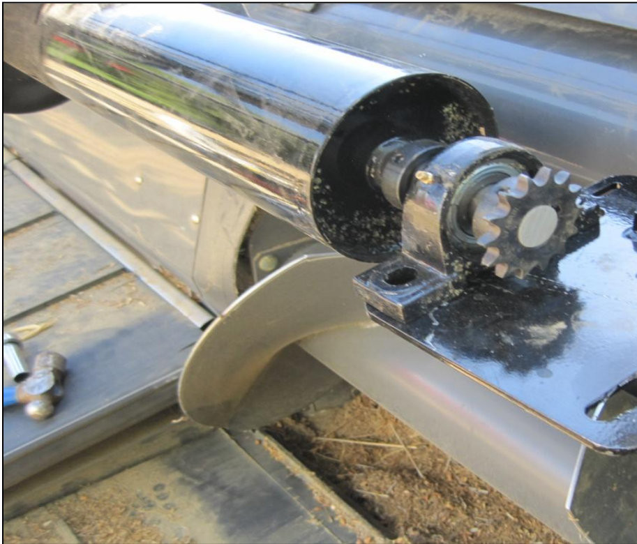
FIG 5 SHOWING AUGER BEARING RESTING ON THE TOP OF THE CENTER BEARING PLATE.
