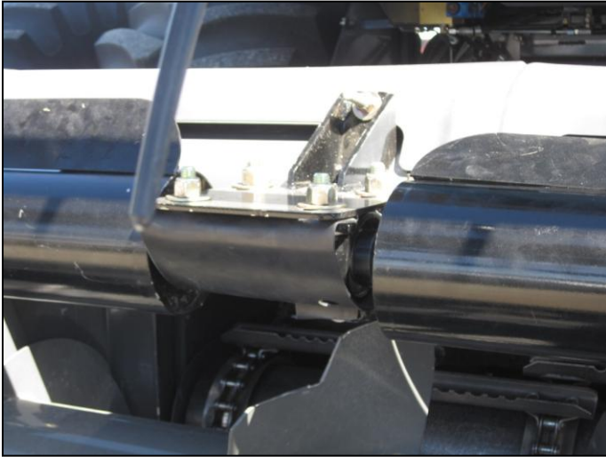
FIG 11 CENTER PLASTIC TO COVER THE BEARINGS AND CHAIN COUPLER.
