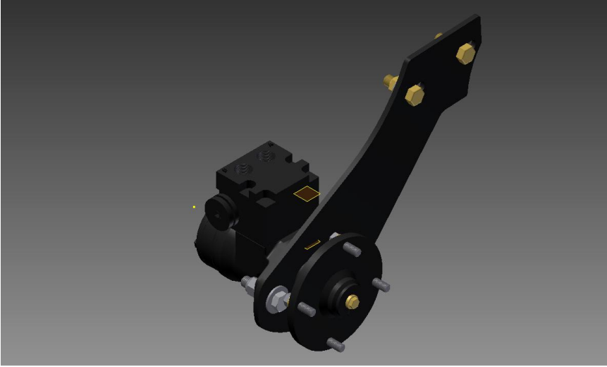
FIG 2 RH END MOUNT WITH MOTOR AND DIRECT DRIVE. SEE 405862 RH END VIEW FOR MORE DETAILED PART BREAK DOWN.
