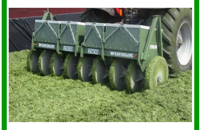
The Weaverline 2900 series Silage Packers are built to help you pack faster and better. With heavier wheels, no lip on the rim and lower boxes for less vision obstruction, the 2900 series packers take the advantages of earlier design Weaverline packers and bring it all together in a machine that helps you pack more effectively, which means more feed and less air in the trench.
