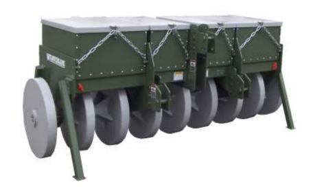
wheel design helps to rake and level the pile when there is excess loose material on top, but the gussets are clear of the pack when proper density is achieved. The Weaverline packer has the outside wheels at the very edge of the machine, making it much easier to get a tight pack right up to the trench wall. The Weaverline Silage Packer is an efficient and very effective packing machine that will help to get consistent density numbers from top to bottom and wall to wall in your trench.
