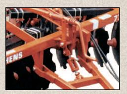
TWO STAGE LEVELING keeps the frame level in the field and in transport. After hitching the clevis to the tractor, the turnbuckle adjusts the tongue position to level the disk frame in transport. In the field, a leveling screw that connects the tongue to the wheel carriages is adjusted for field conditions and discing speed desired. After initial adjustment, the frame remains level while being lifted and lowered. A TURNBUCKLE connects the wheel carriages for precise side-to-side leveling.
