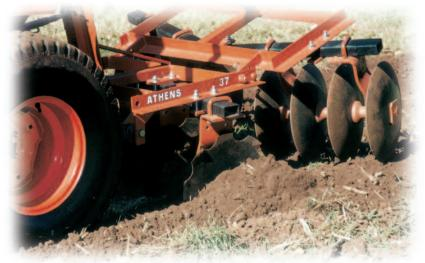
Weight per blade ranges from 35-42 pounds. Above: The Rear Frame is pinned up to increase the weight on the front gangs for the initial pass.
