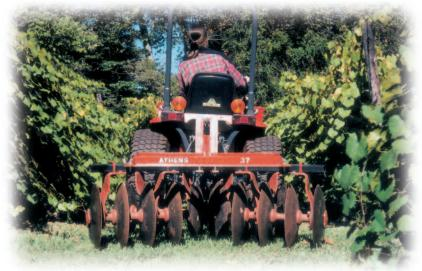
The Athens Model 37 is ideal for orchards and vineyards. Its compact design allows easy lifting, straight pulling and excellent maneuverability in small fields and around close objects.
