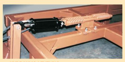
**HYDRAULIC LEVELING** from the tractor seat provides positive control for varying conditions. A set of four strong leveling springs takes the shock out of the leveling mechanism. Whether in transport or operation, front to rear leveling is controlled at your fingertips. (wide frame shown)
