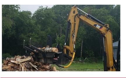
Perfect for residential and farm use, the HWP-120 Firewood Processors truly makes the job hassle-free. When attached to a skid steer or other machine, it enables one person to easily and efficiently perform wood cutting and splitting tasks. All from the comfort of the cab. Take the processor to the wood, instead of having to bring the wood to the processor. The mobility and efficiency of these Firewood Processors is a time saver!
