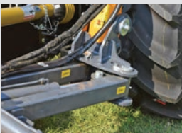
Hydraulic side shift cylinder fitted within the parallel arms for better protection during work.
