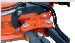
Rotation joint on self lubricating bushing.
