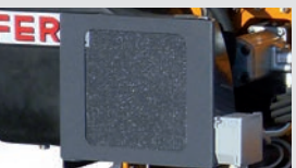
Oil cooler with thermostat (optional)
