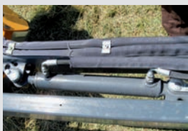
Hydraulic side shift cylinder fitted within the parallel arms for better protection during work
