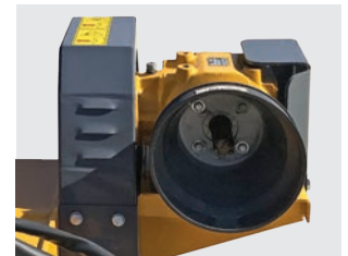
Gearbox unit outside the transmission cover
