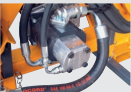
Group 3 cast iron hydraulic rotor pump
