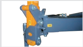
Mechanical breakaway (protection in case of obstacles).
