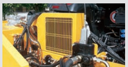
Oil cooler with thermostat
