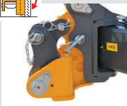
Mechanical locking pin for transportation, (no chains, no brackets).
