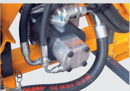
Group 3 cast iron hydraulic rotor pump
