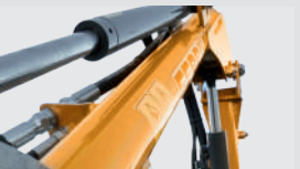
Circular section power arms High Torsion Resistance
