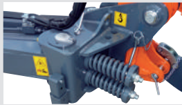
Mechanical breakaway with spring assisted device.
