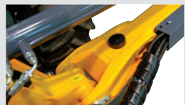
Frame "DELTA BOX" (forces shared and balanced)
