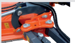
Rotation joint on self lubricating bushing.
