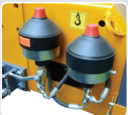
Lift float nitrogen accumulator.
