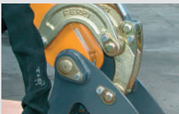
Drop forged lever for flail head rotation
