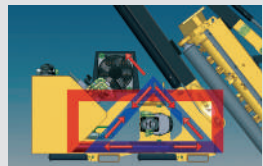
Frame "DELTA BOX" (forces shared and balanced)
