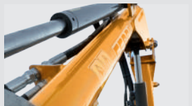
Circular section power arms High Torsion Resistance
