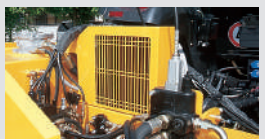
Oil cooler with thermostat
