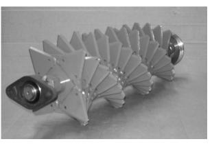
The standard rotor with 76 knives welded to heavy replacement plates which slide easily on the Heavy Duty 1-1/4" Hex Shaft allow for easy replacement of worn blades. Plates can be flipped once to use both edges of the knife.
