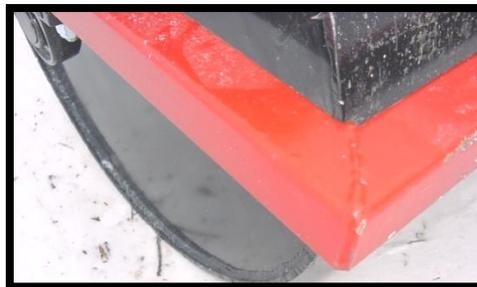
The Extra Heavy-Duty frame is made of 2" square tubing that is 3/16" thick. It has mitered corners and surrounds the drum for added strength. The drum is painted black, and the frame is available in a variety of colours to match your tractor.
