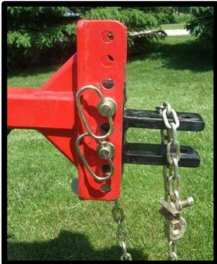
The adjustable hitch clevis has a wide range of settings to accommodate a variety of tractor drawbar heights.
