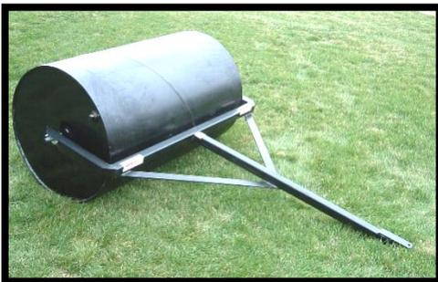
The drum is made from tubular steel 30" in diameter and 3/8" thick. The end plates are 10-gauge steel with 1" bearing on the standard roller. The Extra Heavy-Duty version uses 1/4" steel with 1 3/4" pillow block bearings.
