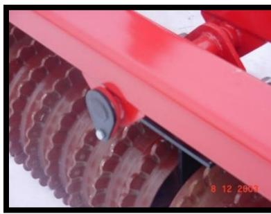
Rugged 1 3/4" hinge pins, securely fastened
