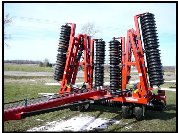
Flex packers are available in a 3-section configuration for widths of 21' to 32' (shown on left). Packers 33' to 50' are built on a 5-section frame (shown right). The balanced frame design minimizes tongue weight.
