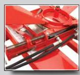
**Hydraulic Shutter** Standard on the XT48, optional on the XT20 and XT24. Operate the shutter remotely with the hydraulic shutter control kit.
