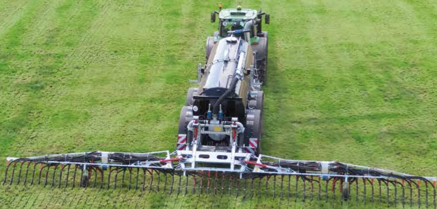
The flow-optimized outlet is a unique feature of the BlackBird, and its design is based on flow simulation data.
