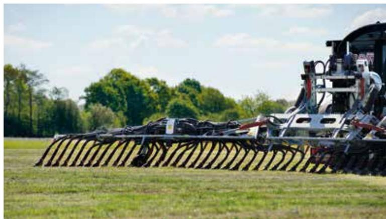
Optimum positioning of precision distributors centrally in boom for improved distribution accuracy
