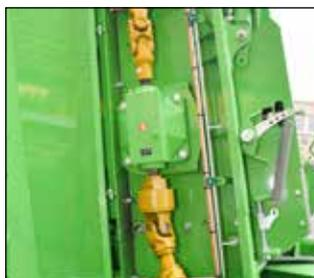
The beaters are driven by P.T.O.-shafts (1,000 rpm) to ensure the safety and the protection of the whole mechanism.
