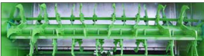
The macerator, fitted with two horizontal beaters with a diameter of 600 mm and with two spreading discs, crumbles and shreds the matter very well.
