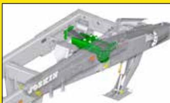
Hitching suspension with parabolic leaves
